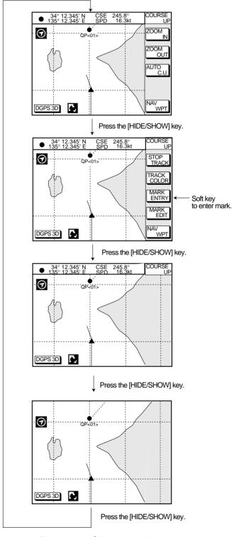
Figure 5-1 Changing displays (PLOTTER display)
